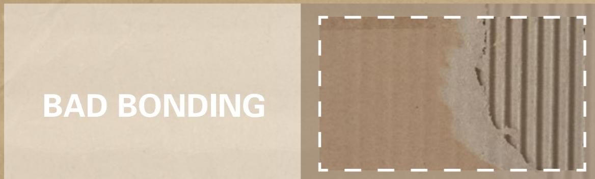
A **low humidity** level prevents the cardboard fibers from opening up and absorbing the **glue properly**. With the **glue remaining on the surface**, it does not enable the **correct bonding** of the cardboard layers.
