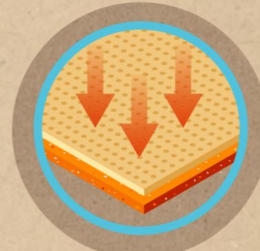
To absorb the **right amount of glue**, the cardboard fibers must be open. This is normally achieved through heat
